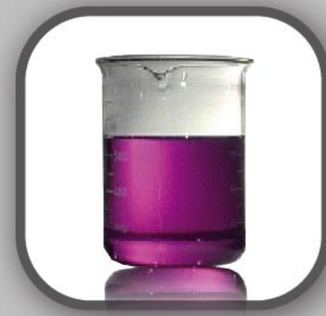
fig. 3: Original, violet color indicates NO organic soiling in the beverage line
