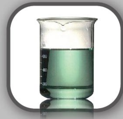
fig. 2: green color indicates organic soiling in the beverage line
